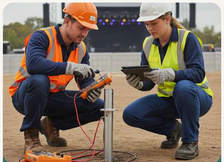
Testing & Documentation: Use 3-point test; add electrodes or treatment if needed
